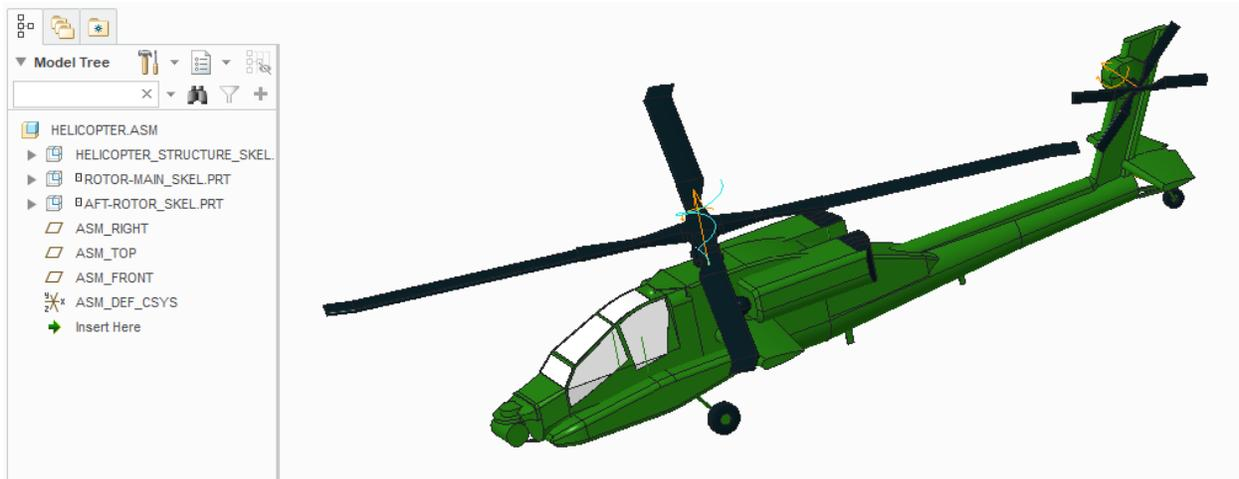
Mechanism captured via multiple skeletons assembled with connections.
